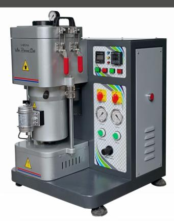
The **Mini Pressure Cost** is a perfect match for small and medium scale jewel smith for quality casting product, invented on special demand from the industry. Metal can be melted under vacuum or inert gas atmosphere. Metal will be poured into the flask with pressure, while there will be high suction vacuum in the flask chamber. Chamber and stopper lift thru pneumatic pressure. Perfect locking and centring of the melting
